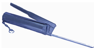
Figure 4 An example of grease gun
